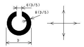
*Figure 1. Landolt's rings. (a) Dimensions (b) Direction of a gap looking from the center of the each ring.*
